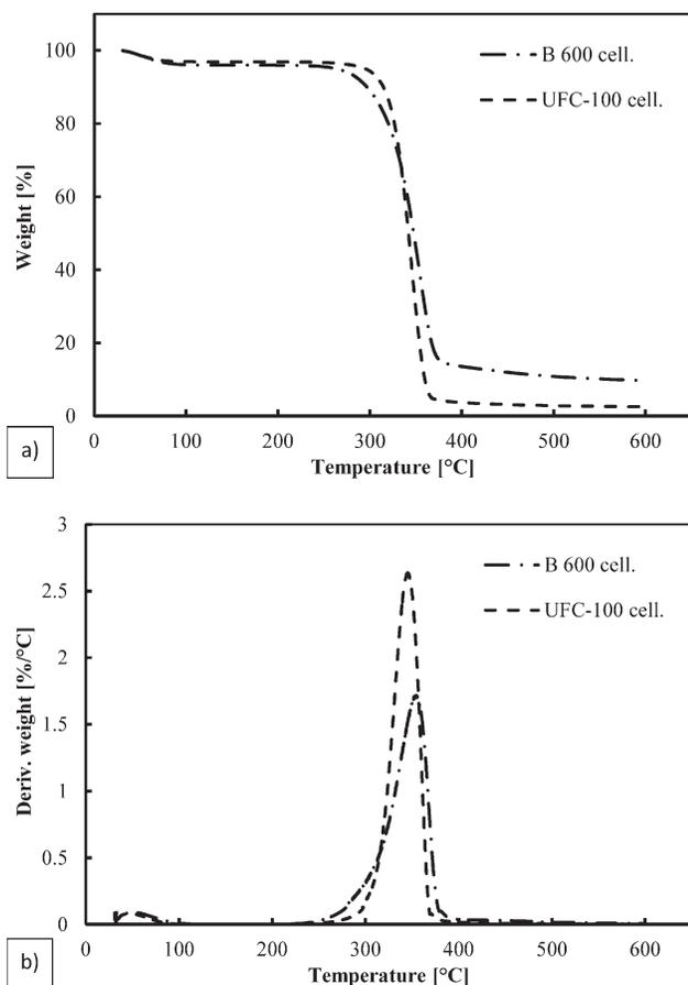
**Figure 6.** TGA (a) and DTG (b) curves of different types of neat MFCs.
