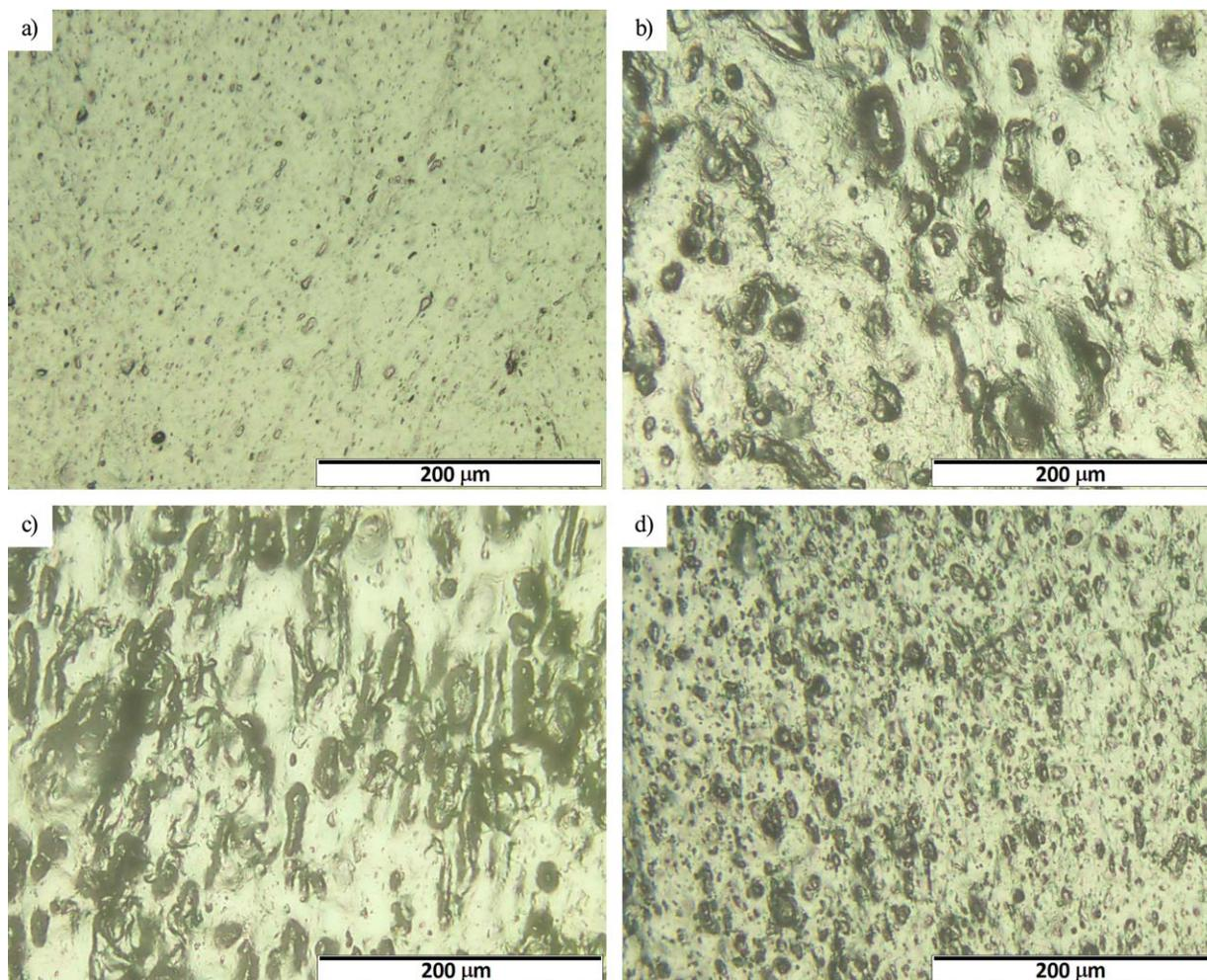
**Figure 4.** OM images taken from the polished surfaces of TPS (a) and TPS/MFC composites (b,c,d). Designations: (a) TPS, (b) TPS\_B600\_10, (c) TPS\_B600\_20, (d) TPS\_UFC\_10. [Color figure can be viewed in the online issue, which is available at [wileyonlinelibrary.com](http://wileyonlinelibrary.com).]
