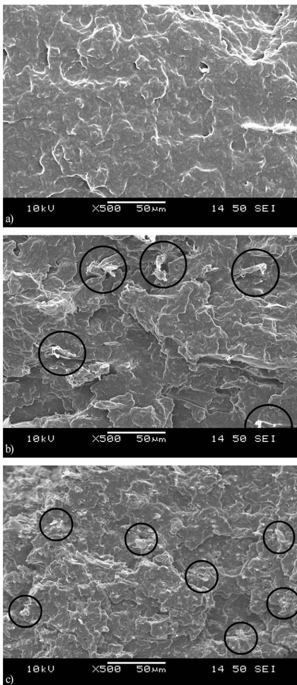
**Figure 3.** SEM pictures taken from the fracture surface of TPS (a) and TPS/MFC microcomposites (b,c). Designations: (a) TPS, (b) TPS\_B600\_10, (c) TPS\_UFC\_10.
