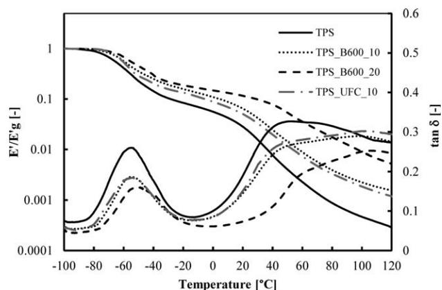
**Figure 5.** Course of the relative storage modulus ( $E'/E'_g$  in semi logarithmic representation) and mechanical loss factor ( $\tan \delta$ ) as a function of temperature for the TPS and its biocomposites with 10 and 20 wt % MFC.
