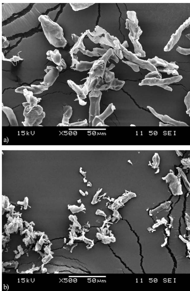
**Figure 1.** SEM images taken from raw MFC particles B 600 (a) and UFC-100 (b).
