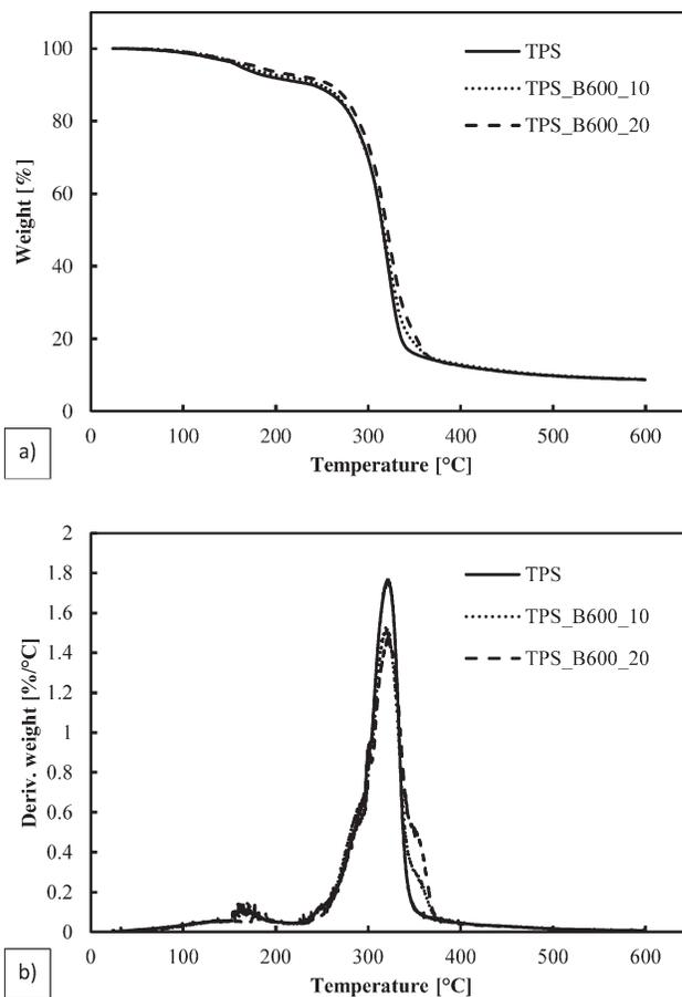
**Figure 7.** TGA (a) and DTG (b) curves of parent TPS and its microcomposites containing different amounts of B 600 MFC.
